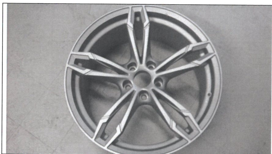
Fig. 1 Sample outsider surface before test start 384h salt spray and rotating bending test
