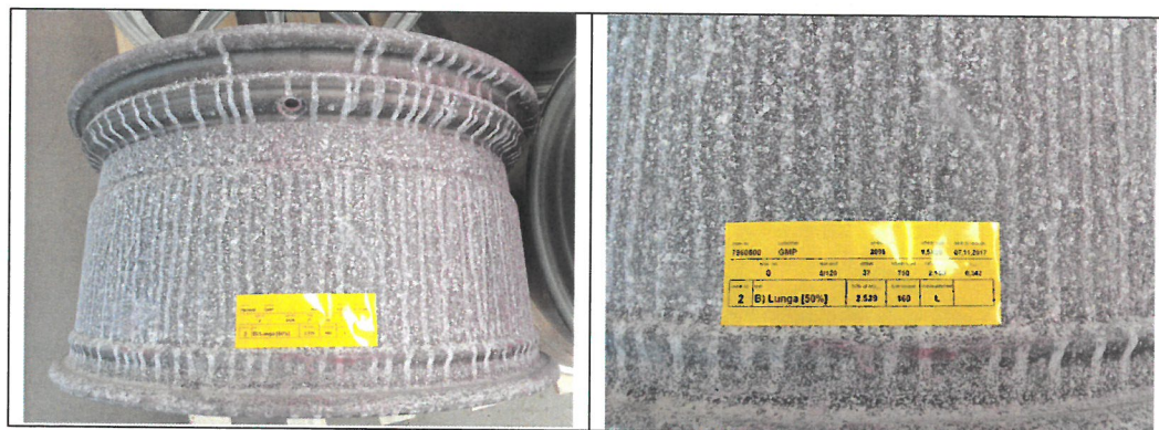
Fig. 2 Formation of corrosion products at the outside surface after 384 h salt spray test
